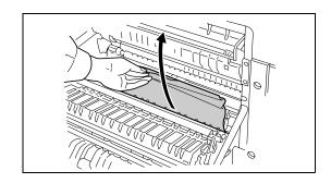
**3** Push the lever (green colored) to raise the duplex unit and remove the jammed paper.
