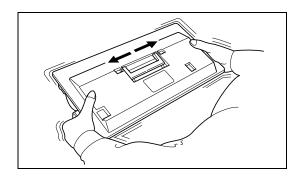
Grasp the handle on the toner container and insert the toner container along the rail of the printer.
