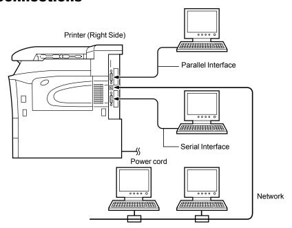
A standard Centronics parallel interface ( ), serial (RS-232C) interface (IOIOI), and a 10/100 base-T connector are located on the right side of the printer.
