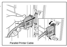
Close the clips on both sides to fix the connector in place.
