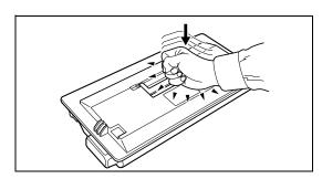
4 Thoroughly shake the toner container (in the directions of the arrows) ten times or more to loosen and mix the toner inside.
