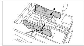
3 Turn the paper stopper located at the right side of the paper cassette to the left as shown and move it to the desired paper size.
