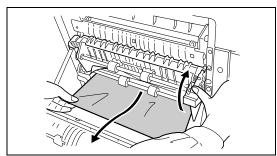
4 If there is jammed paper in the output section, remove it.
