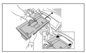
Hold the toner container by hands and fully insert it into the printer.
